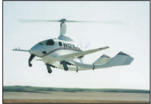
Figure 15-3. The CarterCopter uses wings to enhance performance.
