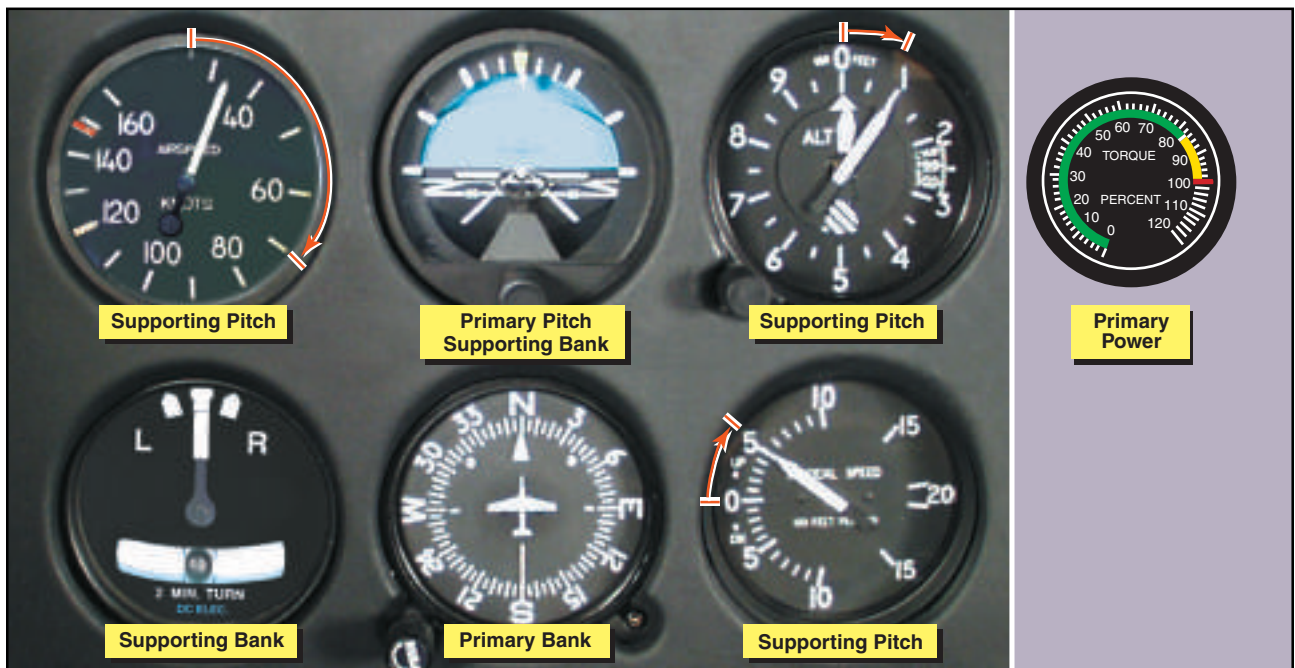
Figure 12-22. Flight instrument indications during an instrument takeoff.
