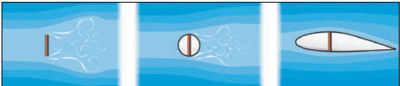
Figure 2-12. It is easy to visualize the creation of form drag by examining the airflow around a flat plate. Streamlining decreases form drag by reducing the airflow separation.
