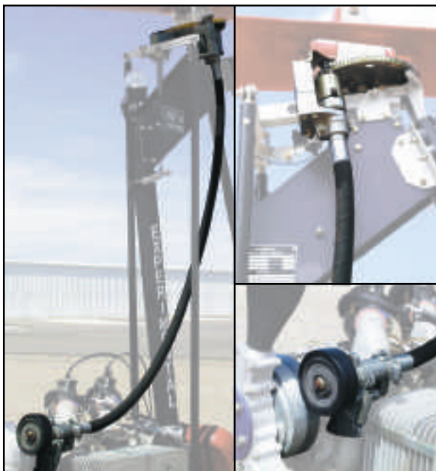
Figure 18-3. The mechanical prerotator used by many gyroplanes uses a friction drive at the propeller hub, and a flexible cable that runs from the propeller hub to the rotor mast. When engaged, the bendix spins the ring gear located on the rotor hub.
