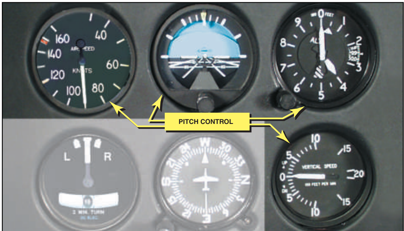
Figure 12-11. The flight instruments for pitch control are the airspeed indicator, attitude indicator, altimeter, and vertical speed indicator.
