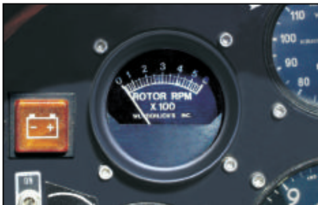
Figure 18-6. A rotor tachometer can be very useful to determine when rotor r.p.m. is sufficient for takeoff.
