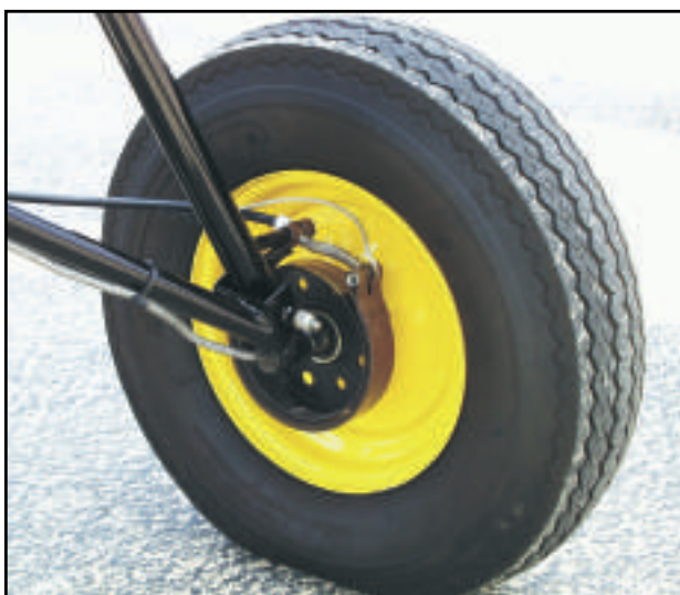
Figure 18-8. Depending on design, main wheel brakes can be operated either independently or collectively. They are considerably more effective than nose wheel brakes.
