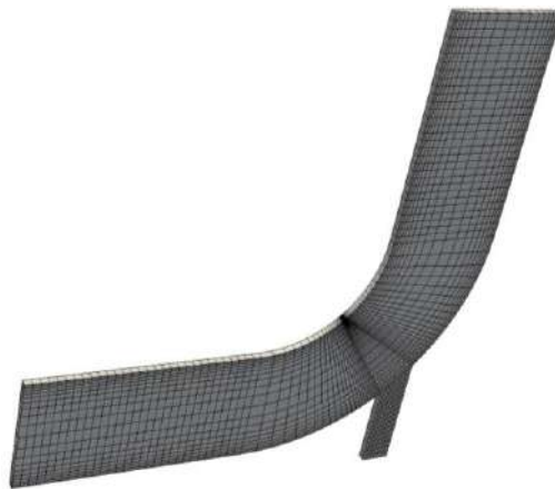
Figure 1.1 The Hex Fine mesh created using GAMBIT
