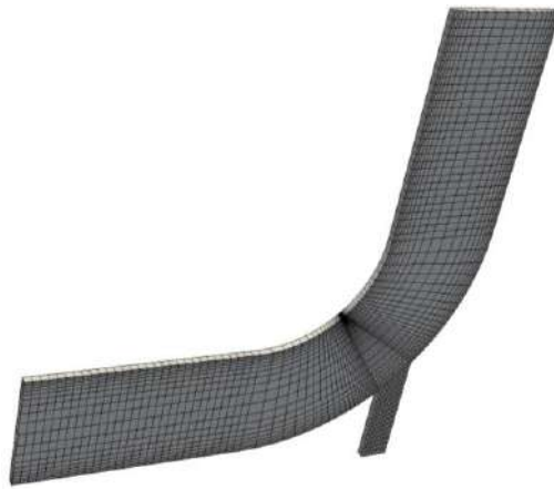
The Hex Fine mesh created using GAMBIT®
