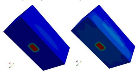
Temperature profile of entire mesh at time 15s and 75s
